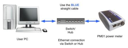
Figure 4 – PM01 connected through a HUB to the NIC in a PC.
