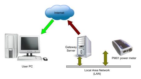
Figure 2 – How the PM01 works.
