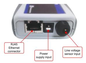
Figure 5 – Location of RJ45, Wall Supply and sensor input connectors.
